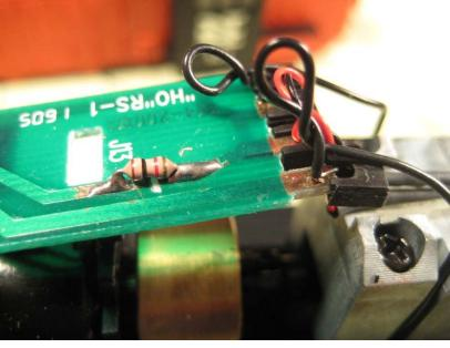
Reconnect wires to like terminals on DCC decoder
